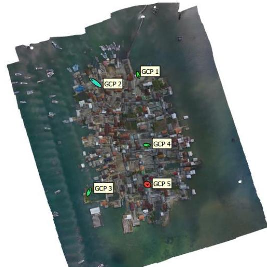
Figure 2. Ground Control Point Distribution.
