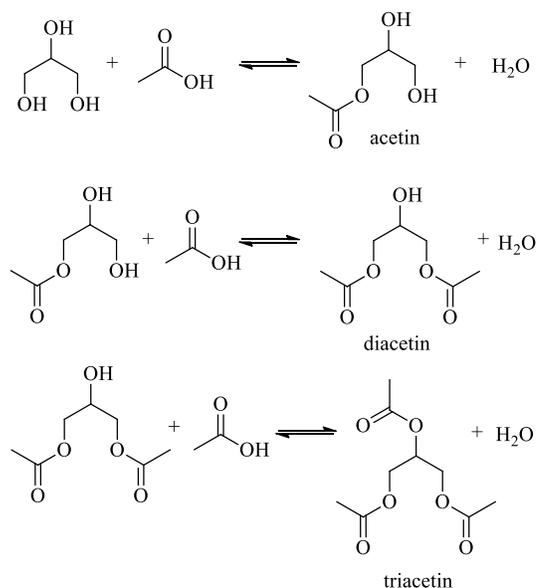
Figure 1. Esterification reaction of glycerol to acetin products.
