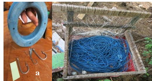
Figure 1. Sharks' fishing gear (a) Fishing line stretching; (b) Basic longline
