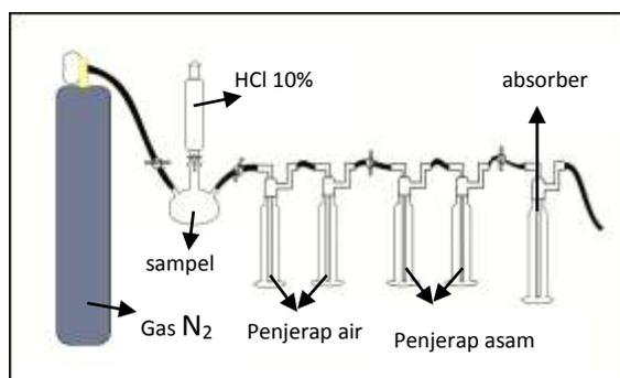
Figure 1. CO<sub>2</sub> absorption circuit
