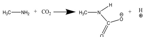
Figure 3. Reaction between methylamine and CO<sub>2</sub>
