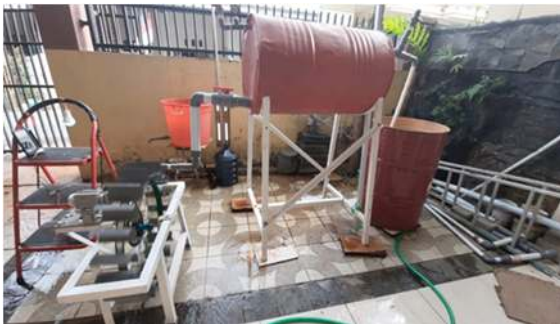
Fig. 5 Prototype form of the Microhydro Gravitational Power Plant
