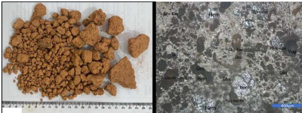
Figure 2. (left) Megascopic appearance of concretion texture of bauxite sample. (right) Petrographic appearance of concretion texture in PPL (Plain Polarized Light).
