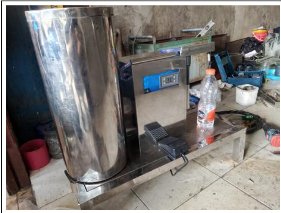
Gambar 7. Mesin Filling Susu ke Standing Pouch .
