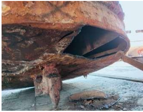
Fig. 1. Corrosion that occurs in the mooring buoy [1]
