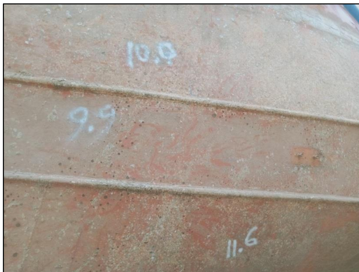
Figure 4. Plate Thickness Test Results
