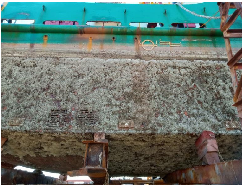
Figure 1. Corrosion on Ship Plates
