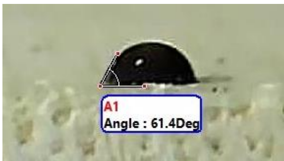
Figure 1. Measurement of the contact angle when liquid penetrates the wood surface
