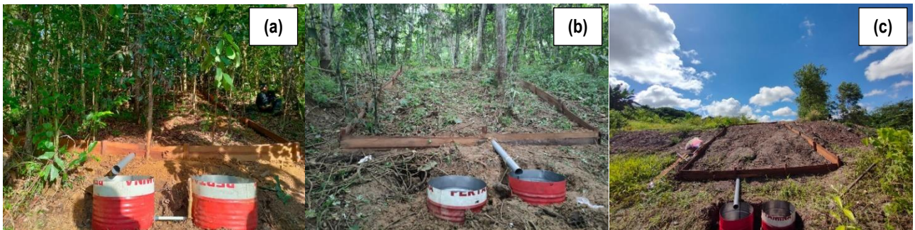
Figure 3. Erosion Measurement Plots (EMP) in A. mangium stand (a), F. moluccana stand (b), and open land (c)
