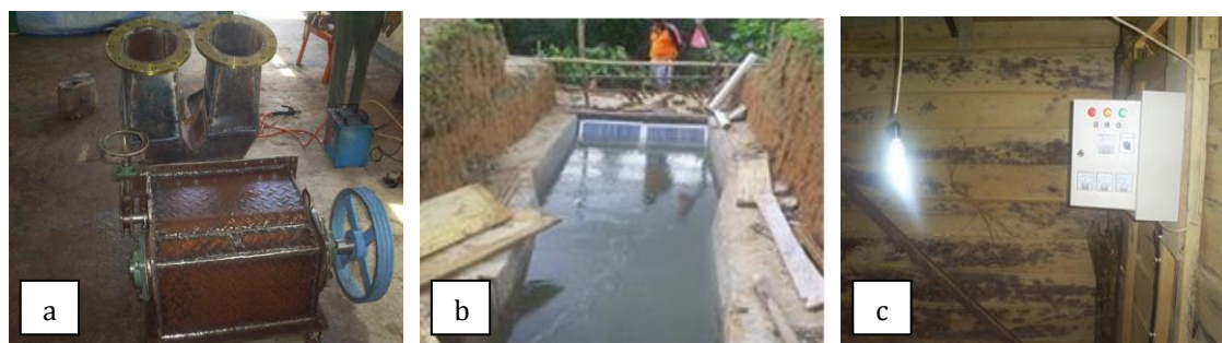
Gambar 2. a. Mesin turbin. b. Bak penampung dan c. Hasil uji coba listrik mikrohidro Figure 2. a. Turbine engine. b. Forebay and c. Electricity trial
