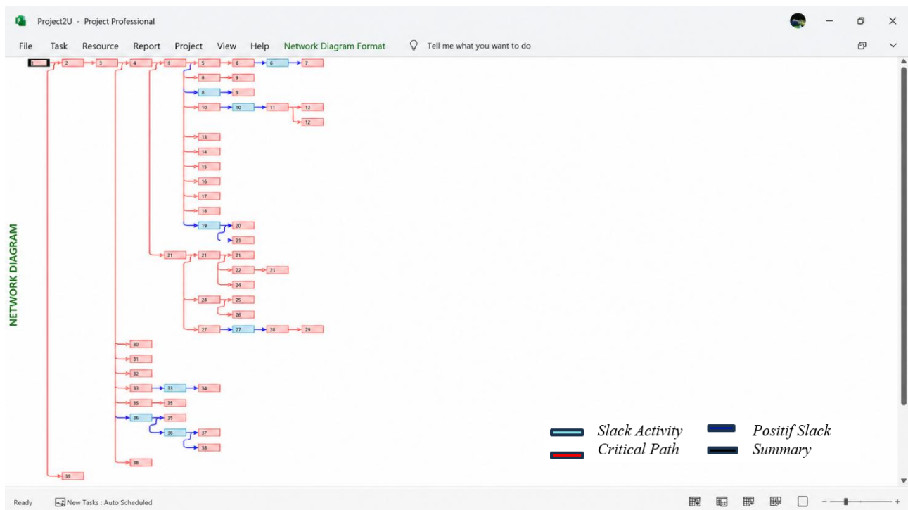
Figure 2. Critical path of the KMP. Kormomolin repair project
